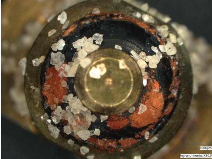
Untreated gasket. You can see that impurities have accumulated on it.
