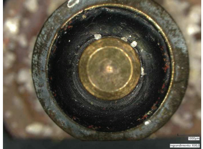
Treated seal. A significant reduction in impurities can be observed.
