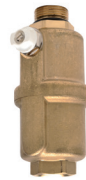
Ball valve for solar systems, for primary circuit of delivery/return piping with built-in thermometer and brass check valve. Seal with cap and gasket, flat seat at one side and G3/4"F on the other side.
