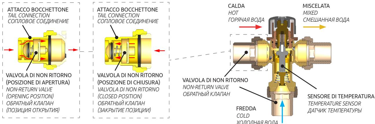
**SCHEMI APPLICATIVI/ APPLICATION DIAGRAMS/ МОНТАЖНАЯ СХЕМА**
