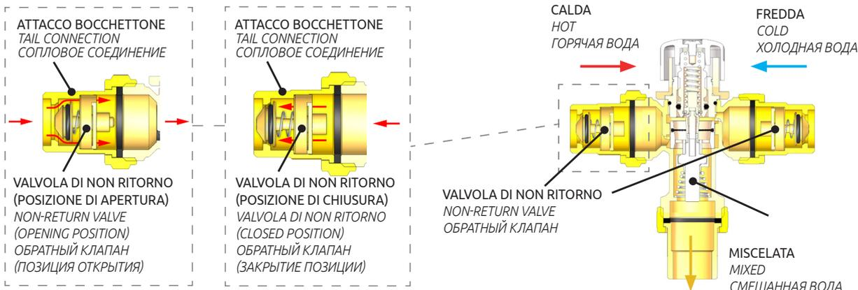
SCHEMI APPLICATIVI/ APPLICATION DIAGRAMS/ МОНТАЖНАЯ СХЕМА
