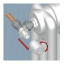
Turn the knob in the counter clockwise direction to remove it com-pletely from the valve.
