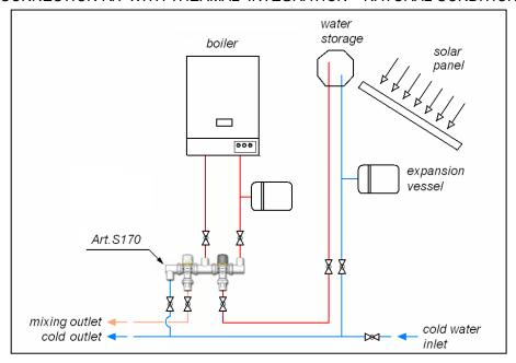
SOLAR SYSTEM WITH PUMP UNIT AND ART.S170 SOLAR STORAGE-TO-BOILER CONNECTION KIT WITH THERMAL INTEGRATION
