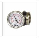
They are specially designed for a simple and safe installation at the head of the manifold bars, they are equipped with a sealing gasket and have a hole for the housing of the thermometers. The supplied thermometers have a reading range of  $0 \div 60^{\circ}$  C.
