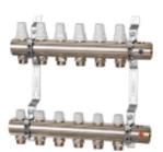
Manifolds unit with adjustment lockshields and valves with thermostatic option. Outlets for 1/2" air vent (art.707) and 1/2" drain cock (art.172). Brackets with anti-vibration supports (art.208). Suitable for 3/4" Euroconus or M24x1,5 fittings. Choose electrothermic actuators with 28x1,5 connection thread.
