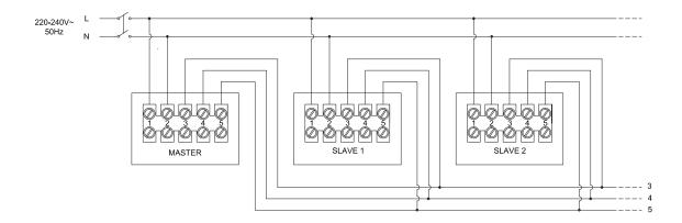
WARNING: Humidity and twilight sensors will detect the values from the first unit connected. In case of a system with long wires or with a lot of electric/electronic equipment may cause signal disturbance to use shielded cables and connect a termination resistor of 120ohm on pin 3 and 4 of the terminal block of the last SLAVE.
