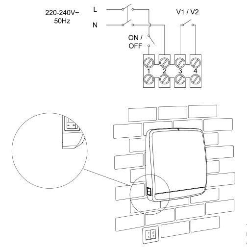
The two switches on the unit must be placed as picture shows.
