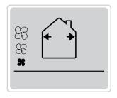
By pressing the specific function button all the units will constantly run in extraction with the possibility to change the speed as required.
