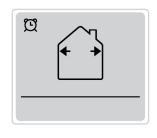
By pressing this button in any of the modes all the products will run in extraction at the maximum speed for 20 minutes, at the end of the cycle they will resume the previous set mode.
