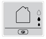
In this mode both humidity and twilight sensors are active, the units will be normally in stand-by with front panel closed, so that when the humidity level in the room exceeds the set threshold the units start running in extraction. Hereinafter explaining how the units run in different situations with related operating mode:
