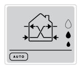
In this mode both humidity and twilight sensors are active, the units will run by themselves without the need to give commands. Hereinafter explaining how the units run in different situations with related operating mode:
