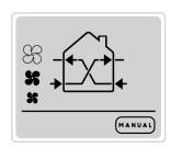
In this mode the sensors are disabled and the units will run with heat recovery. The end user can select the desired speed to run the units and this condition remains until a different command is entered.
