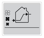
In this mode the units generate a continuous air flow going from MASTER or SLAVE SAME AS MASTER units to SLAVE OPPOSITE TO MASTER excluding heat recovery.
