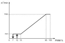
The pumps connected at the outputs PWM E and/or PWM E operate according to the "PWM2" standard, through the solar logic, also known as "normal".
