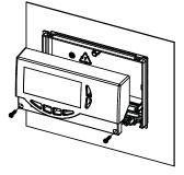
ASSEMBLY WITH CABLE INPUT ON THE LOWER SIDE: fit the cable fasteners and/or the blocks delivered with the unit.
