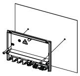
5 Fit the cover again with the electronics at the base.
