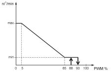
The pumps connected at the outputs PWM E and/or PWM W operate according to the "PWM1" standard, through the heating logic, also known as "inverted".
